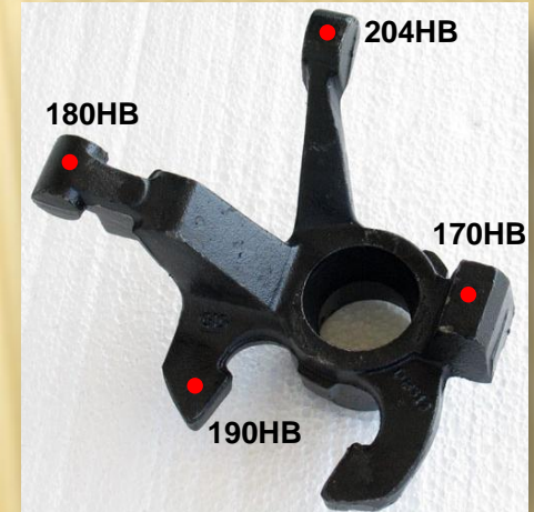
As-cast part with hardness non-uniformity
